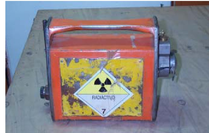
FIG. 2. Industrial radiography container involved in the accident in Cochabamba.
